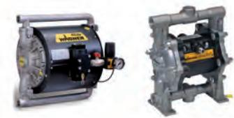
In diaphragm pumps, the material is drawn out of the container via a double diaphragm and fed through hoses or pipes to the spray gun with the necessary pressure. All Wagner diaphragm pumps are double membrane pumps characterized by a material feed with very low pulsation. These pumps can be grouped into simple double diaphragm pumps, ratio double diaphragm pumps and high pressure double diaphragm pumps.
