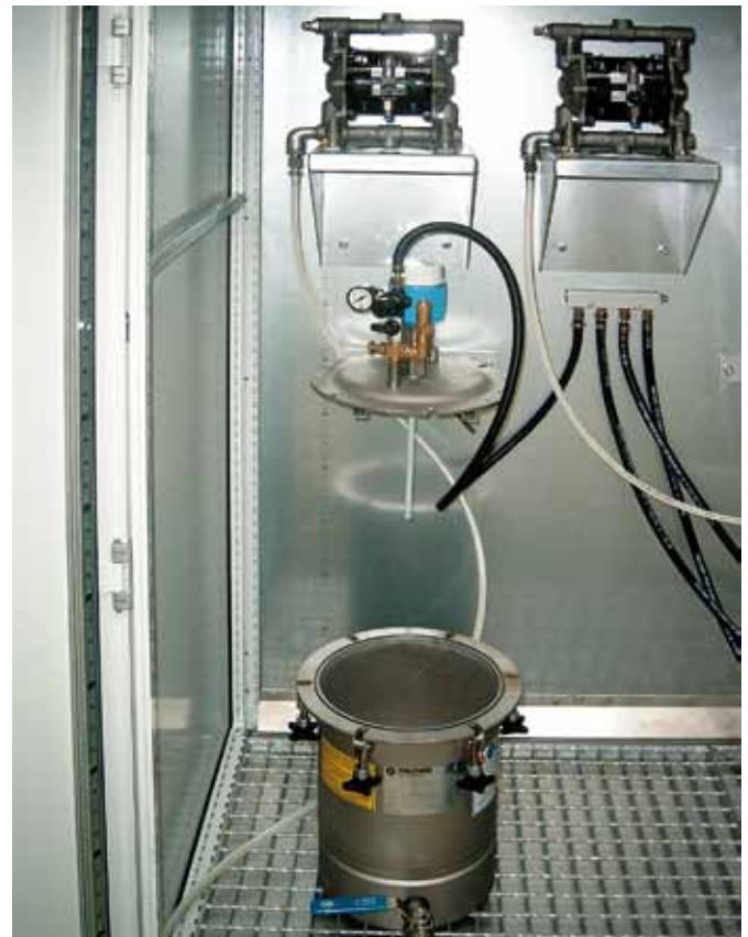
Cabinet with material delivery system (pressure tank with shelf consoles for the cover, dual-diaphragm pump, sump and fill level measurement probe)
