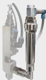
Miniature material pressure tank, 45 ml, 3 bar, made of stainless steel. The tank is mounted directly on the spray gun. See page 4 for the Select 1 System.
