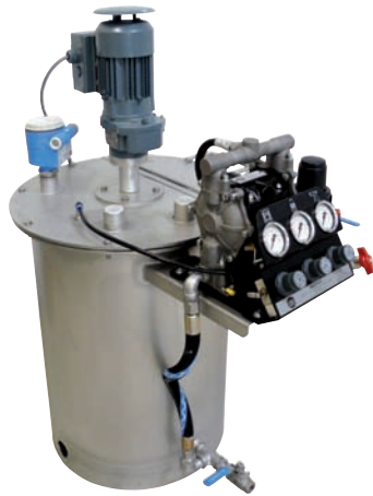
Paint mix tank equipped with pump, agitator and level sensor
