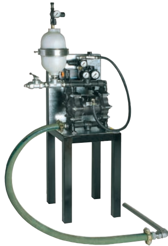
MBP 8034 double diaphragm pump for dispersion adhesives mounted on a "chair". The unit is also equipped with a pulsation dampener, a compressed air fitting and a suction hose. Up to 3 automatic spray guns can be supplied with material.
